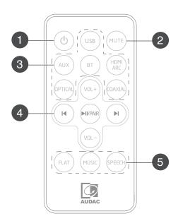
The IMEO2 includes an IR remote controller, which allows the operation of it from a distance of 6 meters.
