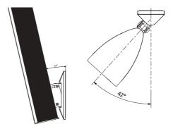
Once installed, the speaker can be can be panned and tilted, focussing the loudspeaker into the desired listening direction. This is useful when the installation height on the wall is limited or the speaker is mounted from the side. The maximum downward tilt is  $13^{\circ}$  and the maximum pan in both directions is  $42^{\circ}$ .
