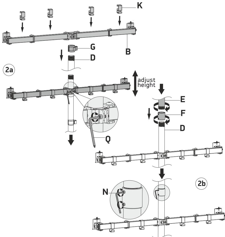
**2c.** Install the plastic hooks (K) onto the upper arm of the bracket (B). Put cable holder (G) on the tube (E). Set desirable height of the arm and tighten screws by using key (Q).
