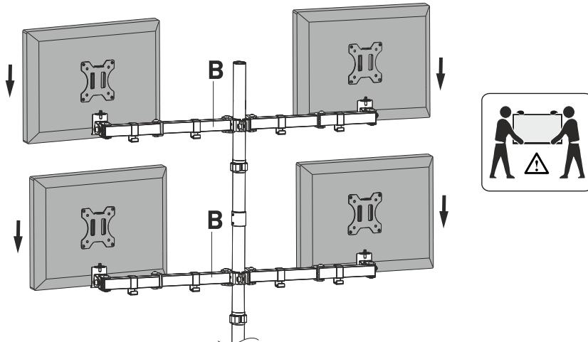
**4b.** Fix VESA-panels (A) with screw (J) through a spacer (I). Install your screens at a desired angle and turn the key (Q) clockwise to tighten the screw. In order to set another angle just loosen the screw a bit.
