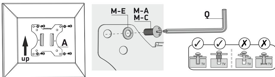
Other screws (M-B), (M-D), washers (M-E) and spacers (M-F) can be used as required. You may use the key (Q). Make sure VESA panels are securely fixed. Look carefully at the picture below.
