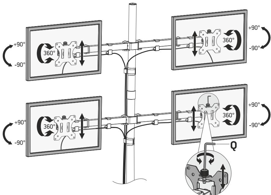
**IMPORTANT:** DO NOT overtighten mounting screws, it can damage the mount and your equipment.
