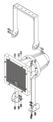
The mounting bracket includes all parts as listed below. Make sure all these parts are included with the delivery to ensure a safe and secure mounting of the loudspeaker.
