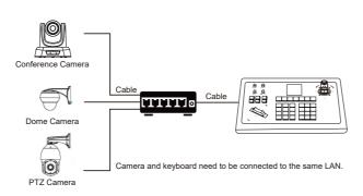
RS485 Control Output: RS485+ of PTZ camera connects to Ta of RS422 on the joystick controller and RS485 - of PTZ camera connects to Tb of RS422 on the Joystick controller
