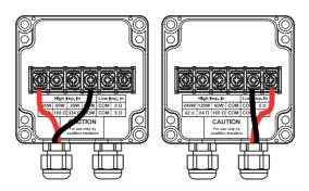
Above image indicates an example for both a 100V (left side) and low impedance (right side) connection example.
