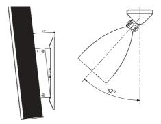
Once installed, the speaker can be can be panned and tilted, focusing the loudspeaker into the desired listening direction. This is useful when the installation height on the wall is limited or the speaker is mounted from the side. Depending on the selected speaker part, the downward tilting angle can be adjusted within a range of 0° and 6.5°, or within a range of 6.5° and 13°. The maximum pan in both directions is 42°.
